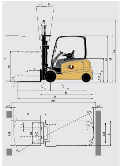
Ast = Working aisle width with load
