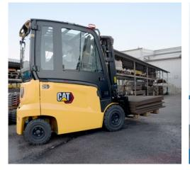
The Cat<sup>®</sup> *Responsive Drive System (RDS)* seems to know how the driver wants the truck to behave at any moment. Reacting to the speed of accelerator pedal and hydraulic control movement, it instantly selects the most appropriate performance mode. *RDS* also smooths out all stops, starts and other actions.
