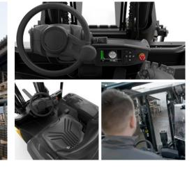
The spacious, high-comfort cabin and its equipment are ergonomically designed to allow strain-free operation with minimal need for the driver to move. Features include a flat, unobstructed floor, adjustable seat and steering wheel, pedals at optimum angles and, to maximise the view, a specially inclined dashboard and counterweight.
