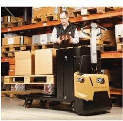
The NPP20N2E is equipped with lifting forks (735 mm height) that offer an ergonomic position for loading and unloading items with minimal physical strain.
