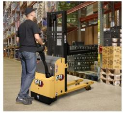
The NPP16PD pedestrian double pallet handler boosts productivity by carrying two pallets simultaneously (one above the other). It is ideal for loading and unloading on dock levellers, picking and refilling, and transporting loads over short distances in warehouses, supermarkets and production areas.
