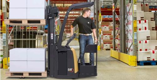
The NPV20PD double pallet handler with foldable platform saves time by carrying two pallets simultaneously (one above the other). It is perfect for double stacking on the loading ramp and for transporting incoming or outgoing loads over short, medium or long distances.
