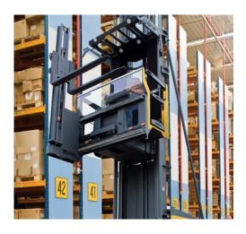
The seven-model NVT range covers lifting heights up to 19 metres\* and capacities between 1.1 and 2.0 tonnes. Thanks to modular engineering, each model can be adapted almost infinitely to meet the specific requirements of your premises and application.
